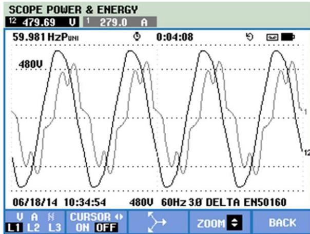
Figure 2 Oscilloscope-picture of line-voltage and -current
