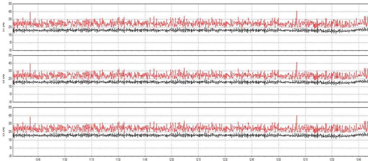
Figure 1 Peak and average kVA-load
