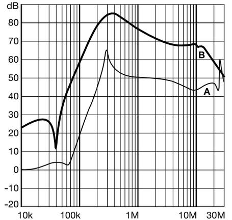
Per CISPR 17; A = 50 Ω/50 Ω sym, B = 50 Ω/50 Ω asym
