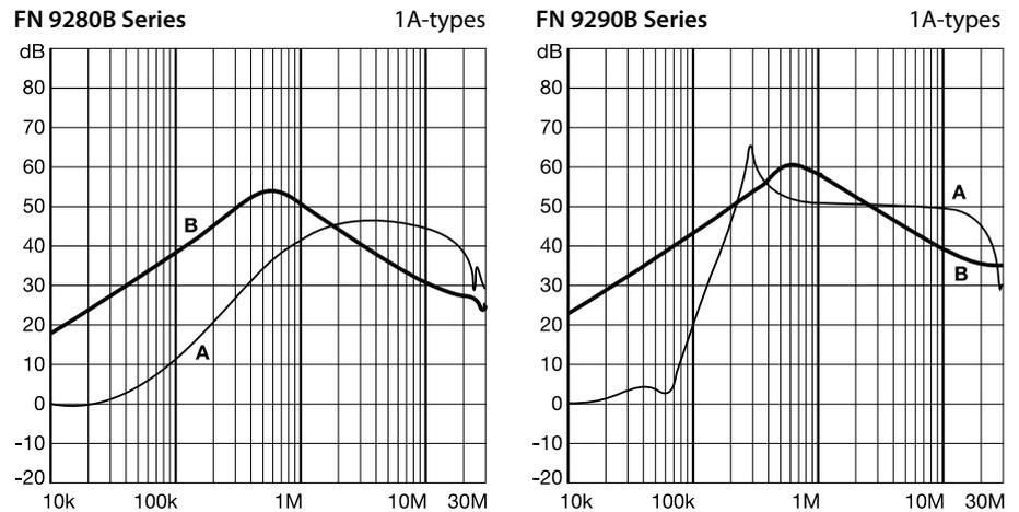
Per CISPR 17; A = 50 Ω/50 Ω sym, B = 50 Ω/50 Ω asym
